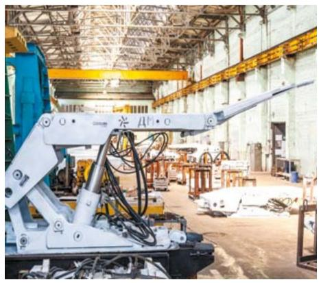
During three months, two sections of powered roof support DM-6.1/15 have been tested and operated together with the previous DM series in the ninth northern longwall of the seam m5 of horizon 450 m in the Dobropolskaya
